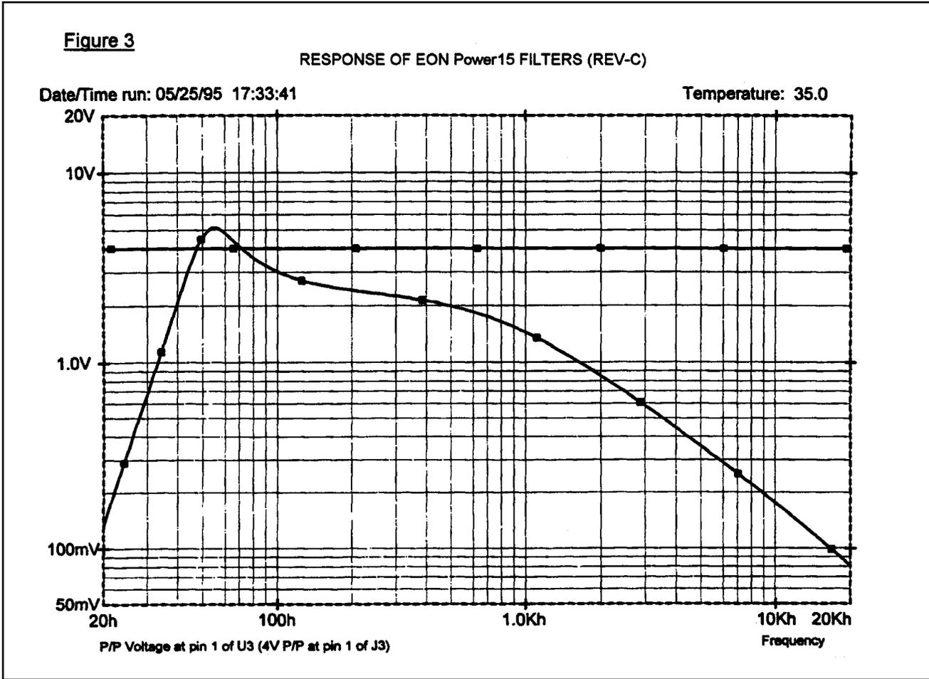
Measure the response at pin 1 of U3. Note in figure 3 above that the input voltage has not been changed. (Voltage at pin 1 of J3). The other curve represents the response at the output of the third section of the filter.
