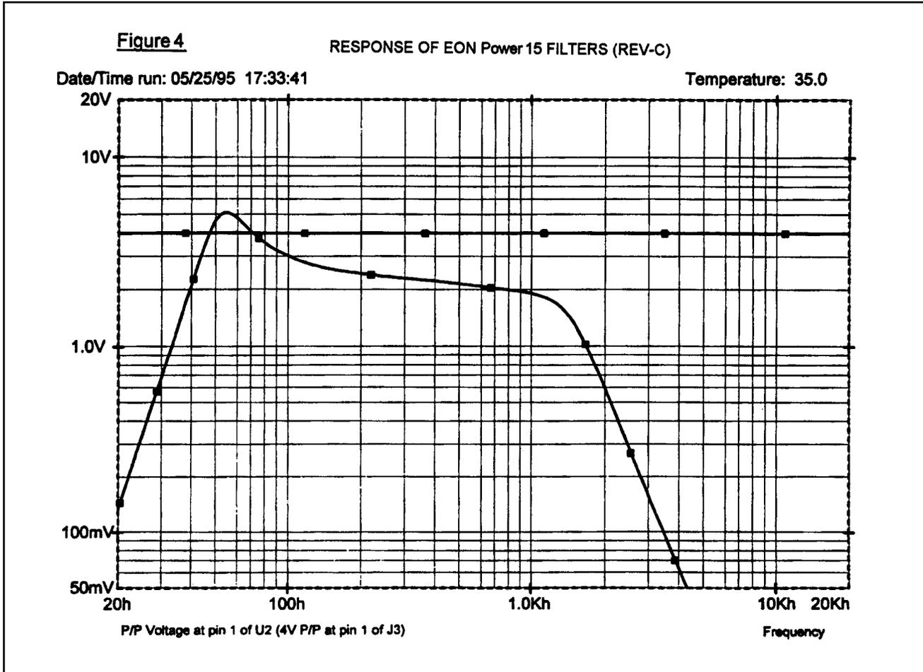
Measure the response at pin 1 of U2. Note in figure 4 above that the input voltage has not been changed. (Voltage at pin 1 of J3). The other curve represents the response at the output of the fourth and final section of the filter. The output is fed to the low frequency power amp that essentially has a flat response from 20Hz to 20kHz.
