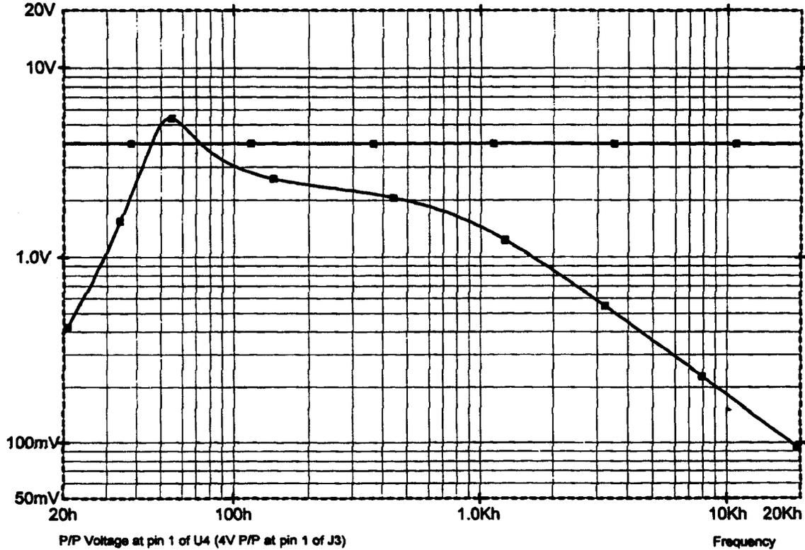
Measure the response at pin 1 of U4. Note in figure 2 above that the input voltage has not been changed. (Voltage at pin 1 of J3). The other curve represents the response at the output of the second section of the filter.
