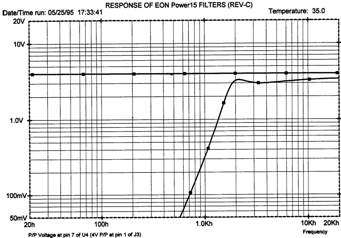
Measure the response at pin 7 of U4. Note in Figure 6 above that the input voltage has not been changed. (Voltage at pin 1 of J3). The other curve represents the response at the output of the second section of the filter.
